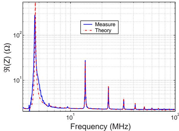
**Fig. 6.** Real part of the electrical impedance of the PZN-7PT plate in a large bandwidth: experiments in solid line, dashed line is calculated from the properties deduced from the fit on the 5<sup>th</sup> harmonic.
