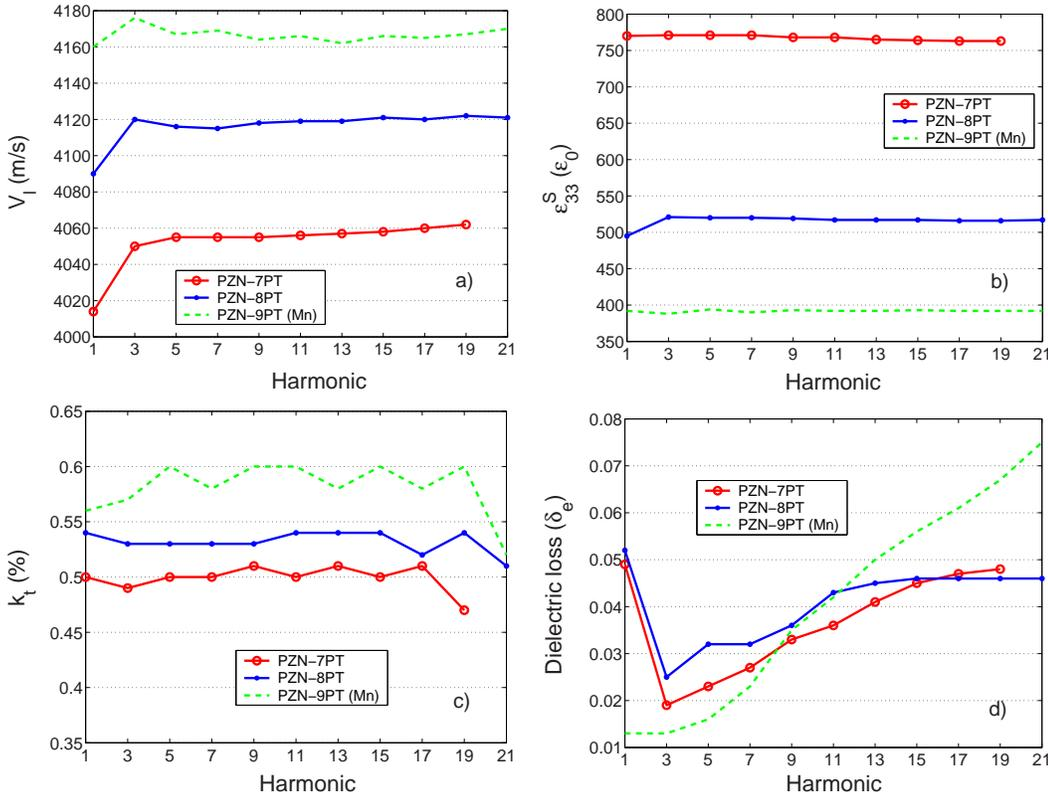
**Fig. 5.** Evolution, with the harmonic order, of the longitudinal wave velocity (a), the clamped dielectric constant  $\epsilon_{33}^S$  (b), the electro-mechanical coupling coefficient  $k_t$  (c) and the dielectric losses (d).
