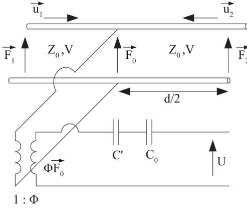
**Fig. 1.** KLM one dimensional equivalent electrical scheme for a piezoelectric material.
