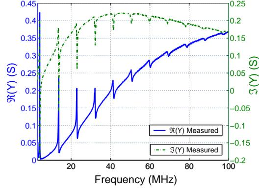
**Fig. 2.** Real and imaginary parts (solid and dashed line) of the electrical admittance of the PZN-7PT plate from the fundamental resonance to the 21<sup>th</sup> harmonic.
