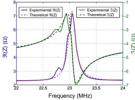
**Fig. 3.** Real and imaginary parts of the electrical impedance around the 5<sup>th</sup> harmonic of the PZN-7PT plate (solid lines: experiments; dashed and dash dot lines: computed curves).
