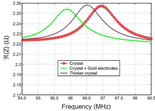
**Fig. 4.** Influence of a 2  $\mu\text{m}$  error on the thickness (solid line) or of 1  $\mu\text{m}$  gold electrode on each face (crosses) on  $\Re(Z)$  computed around the 21<sup>th</sup> harmonic of a 440  $\mu\text{m}$  thick PZN-7PT plate (circles).
